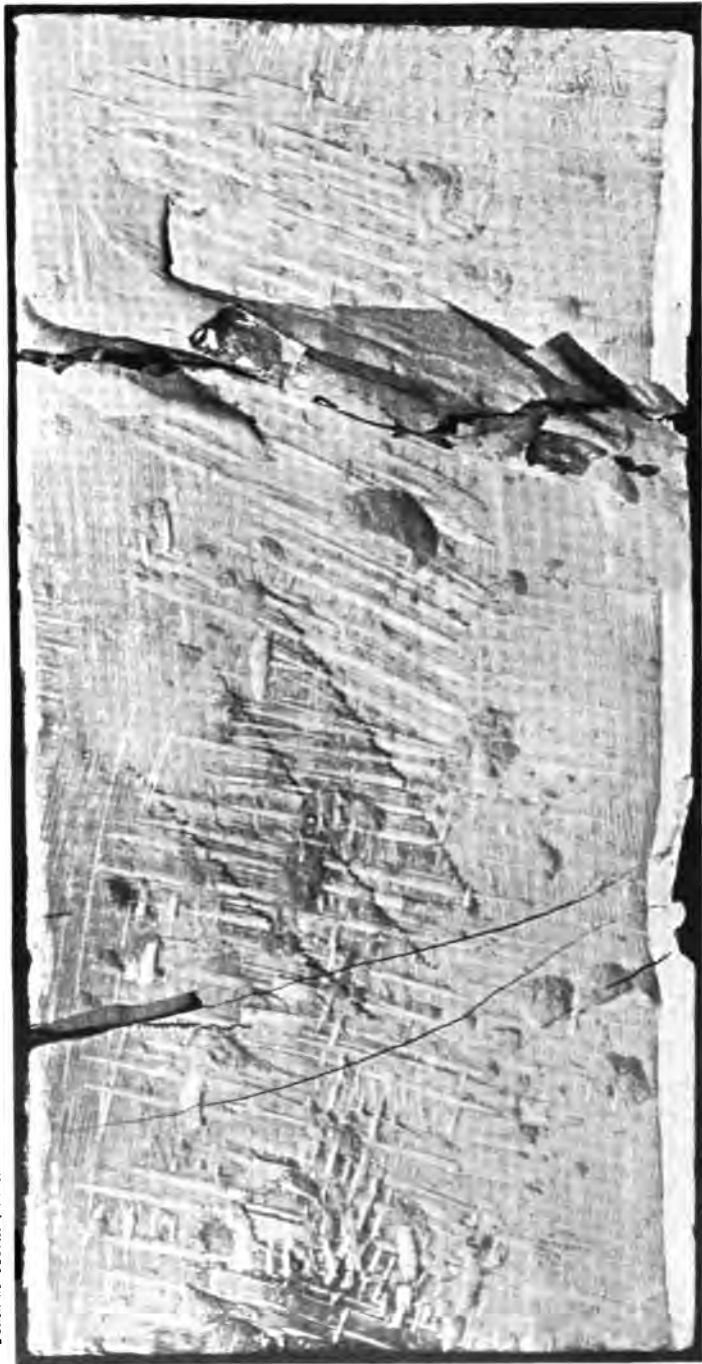
THE SHEARING STRENGTH OF STONES. Photograph of fractured specimen of limestone from Mount Vernon, Ky.
